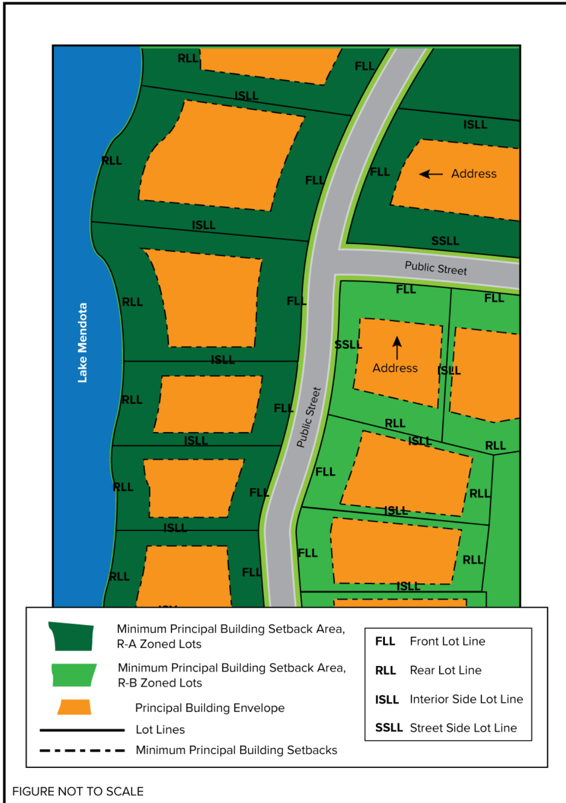
Figure 225.2.3: Illustration of Minimum Principal Building Setback Areas (by Yard) and Building Envelopes for Different Lot Scenarios
